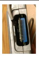
Once you have properly mounted the chip, secure the chip to the ECM with a piece of package sealing or duct tape.
