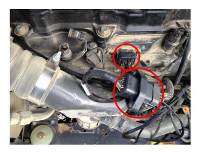
**3)** Locate the MAP Sensor. It is on the same side of the engine as the air intake and it will be closer to the "Fan side" of the engine.
