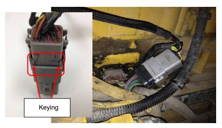
3) The MAP Sensor is on the same of the engine as the air intake, and will be closer to the fan side of the engine. Note: You will need to check for which MAP Sensor is on the engine. If it is a rectangularshaped connector, proceed to Step 4.If the MAP Sensor is a triangleshaped connector, proceed to Step 6.
