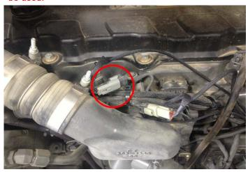
**5)** Plug the male connector from the Ag Diesel Solutions harness to the stock MAP Sensor. Plug the female connector from the Ag Diesel Solutions harness to the stock connector removed from the MAP sensor. Proceed to step 7.
