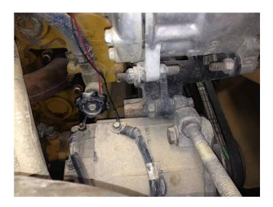
7) Plug the Harness into the module. Mount the module with supplied zip ties away from any excessive heat or moving parts. Note: Zip tie the module to the factory wire harness. Mounting the module with the switch connector down will help prevent moisture from collecting into the module connector
