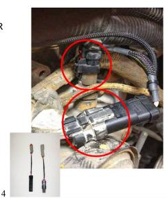
**4)** Unplug the Stock MAP Sensor and then Proceed to Step 5. Note: If your MAP sensor is the same style as what is shown in the below picture, the MAP Sensor jumpers supplies with your module will not be used.
