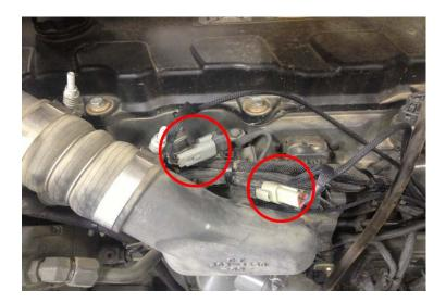
**6)** If the MAP Sensor on your engine is a rectangular-shaped connector, you will need to use the MAP Sensor Jumpers supplied with your module. Connect them in-line between the module harness and Stock connectors.
